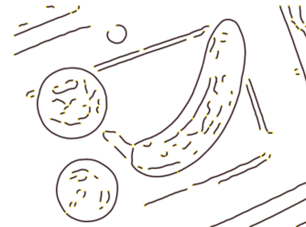
Edge strength |\nabla S| after NMS and thresholding
